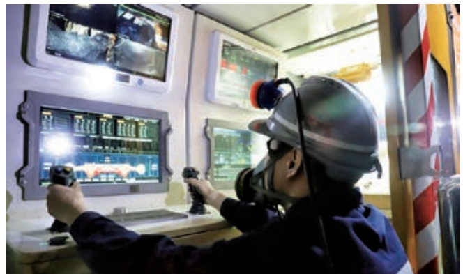
Underground mobile intelligent control room
