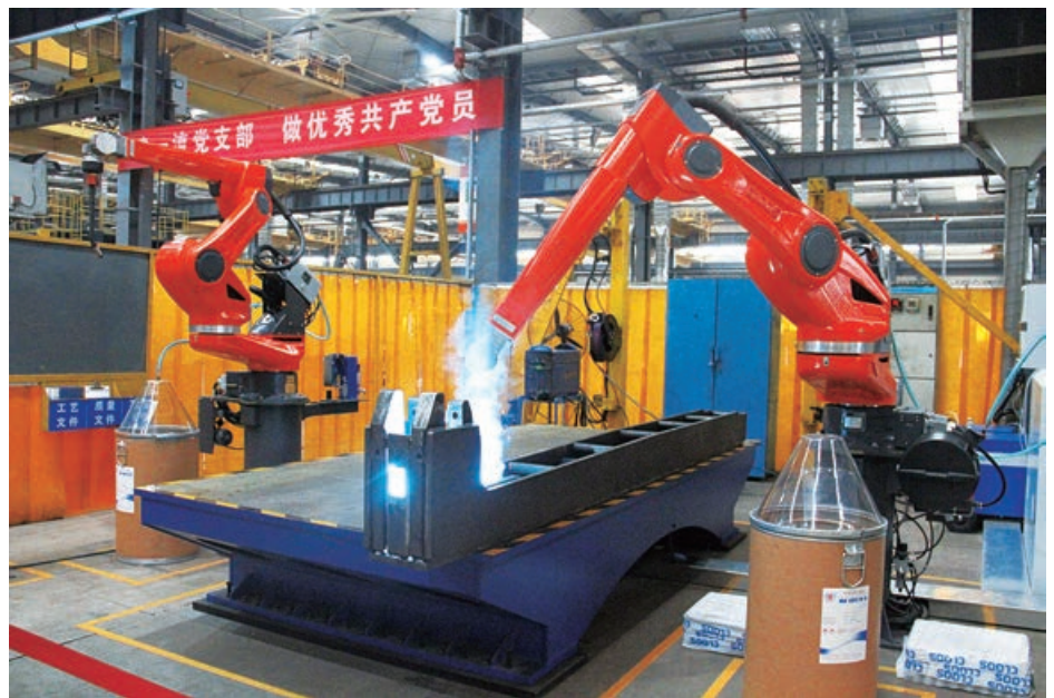
Automatic welding robot
